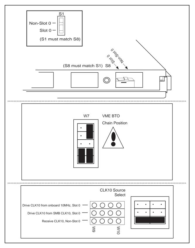
Figure 2-5. VXIbus Non-Slot 0 Configuration
