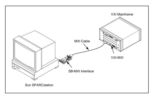
Figure 2-8. MXIbus Single-Ended Cable Configuration
