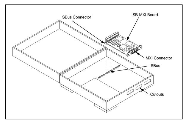
Figure 2-1. SB-MXI Installed in a SPARCstation 1+
