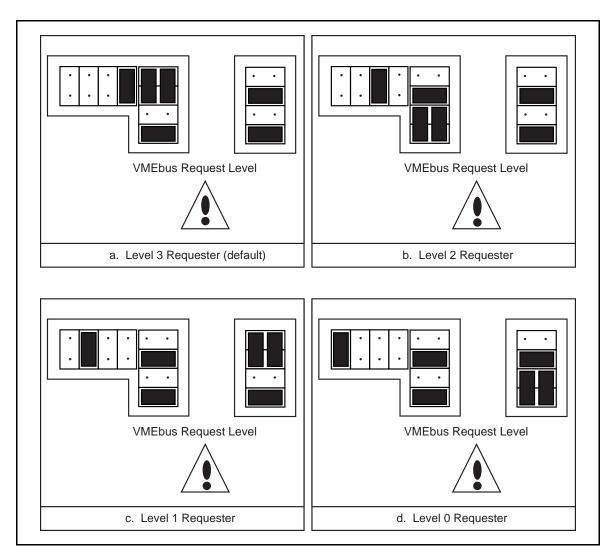
Figure 2-7. VXI-MXI VMEbus Requester Jumper Settings
