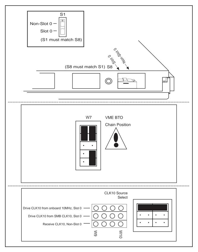
Figure 2-4. VXIbus Slot 0 Configuration
