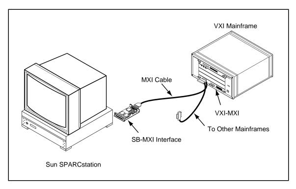
Figure 2-9. MXIbus Dual-Ended Cable Configuration
